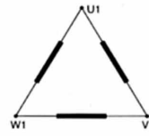
Collegamento Δ Connection Δ Connection Δ
